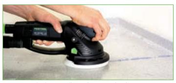
For removing dried excess adhesive from mineral surfaces.
