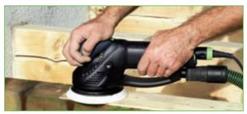
For coarse sanding of weathered beams.
